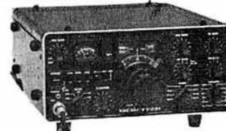
FT221R 144/8MHz, -6 + 1.6MHz shift 10W (plus) SSB, CW, FM, AM, 230/12V
