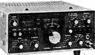
FT620B 50-52 or 50-54 SSB, AM, CW, Ideal transverter source
