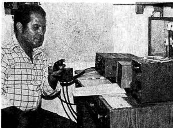
Andy Panayiotou, 5B4BM, CARS contests and awards manager. Active on all bands 80-10m using an FT200 with a wide range of home-brew antennas from verticals for the lower frequencies to monobander beams for the higher frequencies. All these antennas are connected to an antenna exchange unit just visible on the wall behind 5B4BM
