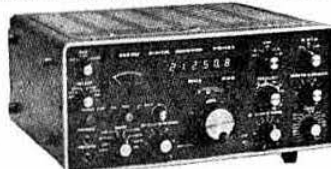
FR101D 160-10m, 2 and 4m, BC bands, FM, SSB, AM, CW
